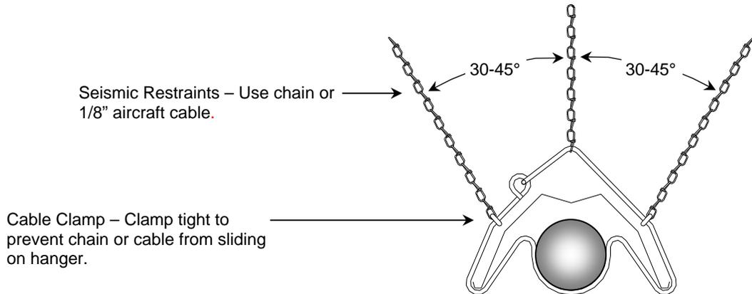
**SEISMIC SUSPENSION FOR HIGH WIND OR OUTDOOR APPLICATIONS**
