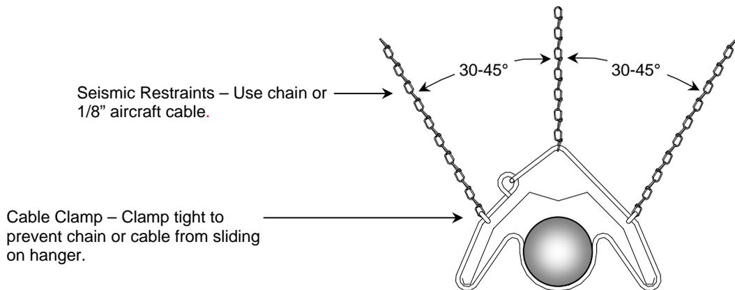
**SEISMIC SUSPENSION FOR HIGH WIND APPLICATIONS**
