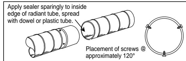
2. Secure joint with sheet metal screws to provide a mechanical joint rather than rely on friction. Use damp cloth to remove excess sealer. Heat tube and fitting assembly ends are designed for minimum clearance and tight fitting to minimize air infiltration.
