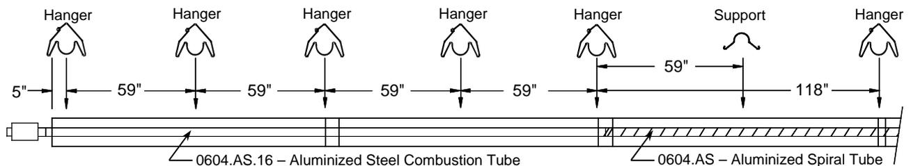
**INSTALL COMBUSTION TUBE WITH WELD SEAM ON BOTTOM**
