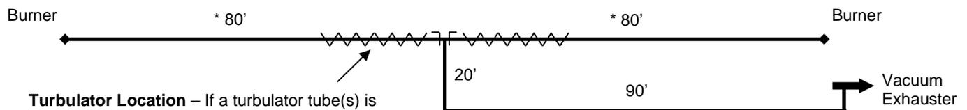
**Turbulator Location** – If a turbulator tube(s) is supplied with the system, it must be installed before the TEE. **DO NOT** install turbulator tube in the common radiant tube after the TEE.
