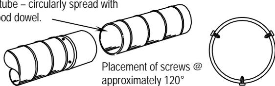
2. Secure joint with self-drilling sheet metal screws supplied. Use damp cloth to remove excess sealer.
