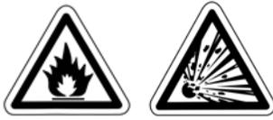
Placement of explosive objects, flammable objects, liquids and vapors close to the heater may result in fire, explosion, death and serious injury or property damage. Do not store or use explosive objects, liquids and vapor in the vicinity the heater.
