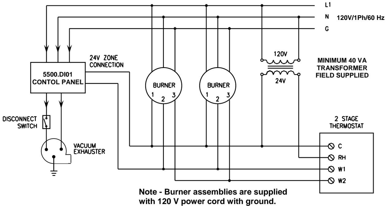
This control panel, associated burner(s) and vacuum exhauster MUST be on the same circuit.
