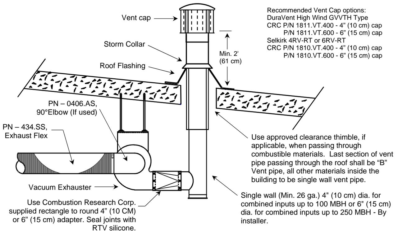
**For the following system lengths, which are classified as ‘Category I’ venting, use appropriate venting materials rated for 550° F (288° C). Do not use Type B Vent;**
