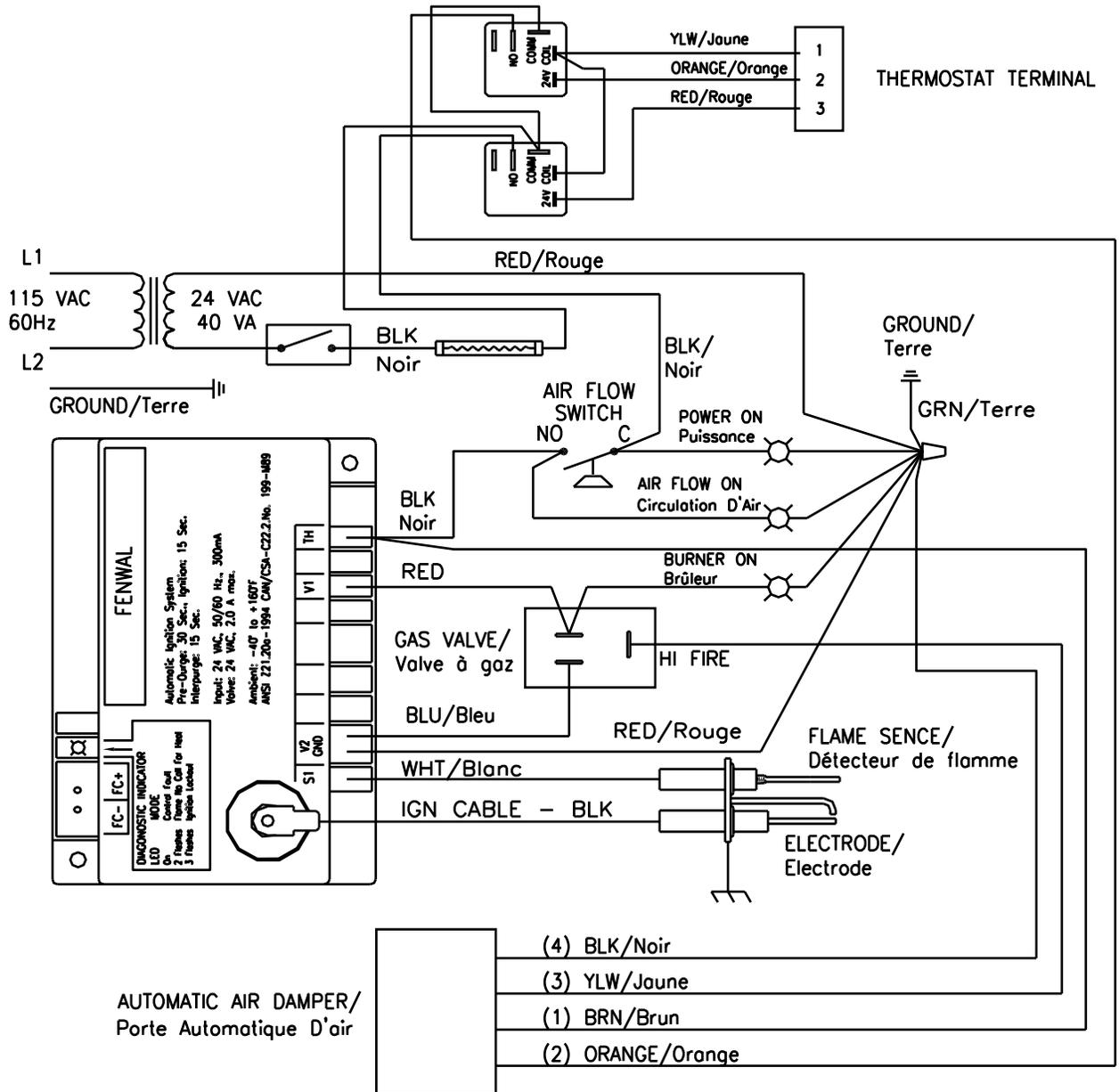
**OPTIONAL SINGLE BURNER WITH INTERNAL WIRING DIAGRAM**
