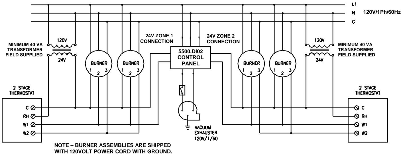
This control panel, associated burner(s) and vacuum exhauster MUST be on the same circuit.
