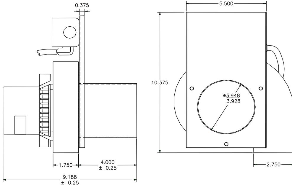
**NOTE** - Motor substitutions can occur, always refer to the motor manufacturer nameplate for electrical information and wiring instructions. Housings and inlets for 0101 vacuum exhauster made with stainless steel are also available – the last two-digit designation will be SS.
