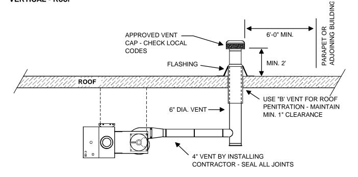
NOTE: VENT PIPING SHOULD NOT EXCEED A MAX. COMBINED LENGTH OF 20'
