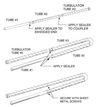
3. Next secure joints with the self drilling and taping screws provided (use three per joint).
