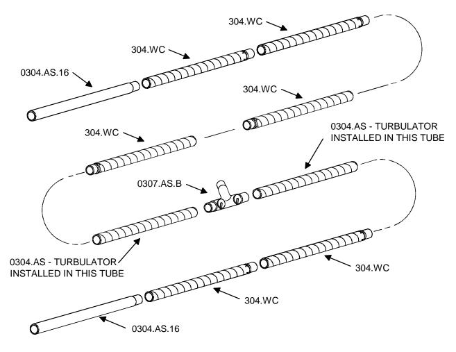
NOTE: Connect the lower Btu/Hr input burner (105,000 Btu/hr) to the shorter length of radiant tube (40' side).
